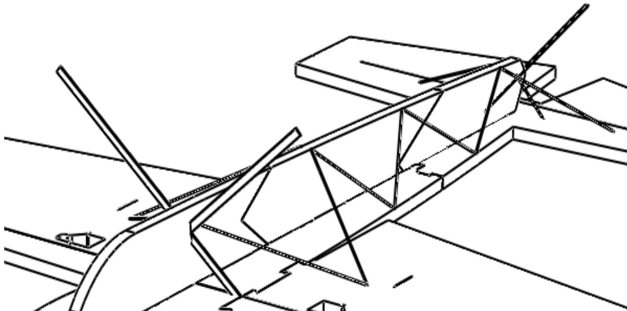
Install your servos, but do not yet glue. With servos in place power them up and install servo arms. Use a straight edge to cut slots in the control panels for the control horns. The Elevator Control Horn will need the slot cut near the Vertical Fuse.
