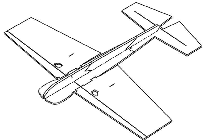
Cut and glue in the 1mm round carbon stiffeners. The placement and lengths are shown on the picture to the right. Start at the gear leg intersection. Use a square to keep all parts perpendicular as you go. It is important that the fuse is straight and square for this step.
