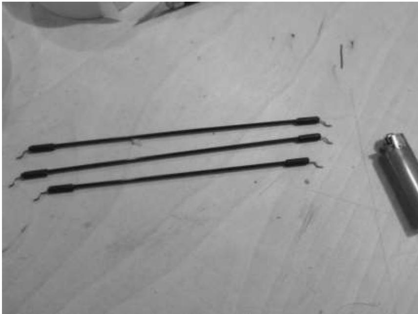
Cut the wire to 1" lengths, you will need 6 pieces. Put a Z-bend onto one end of each wire. The adhesive shrink wrap will also need 6 pieces, but at 9/16" lengths. 2mm carbon tube should be cut to lengths of 7", 7" and 5.5". With the carbon cut attach the wire Z-bends to the tubes by heating the shrink wrap around them.
