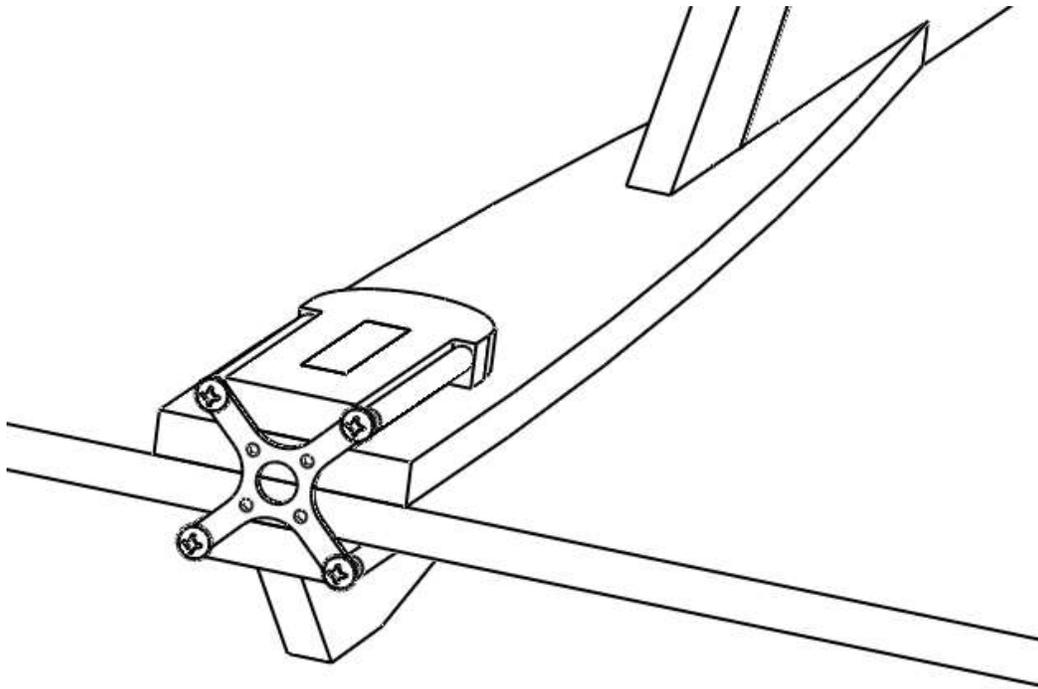
Place the long foam part over the tab sticking thru the bottom of the plane. Then slide the upper motor mount onto that. Check the alignment of the plastic tubes to your motor mount. For a 28mm pattern the tubes will be flush to the foam side up on the top down on the bottom.
