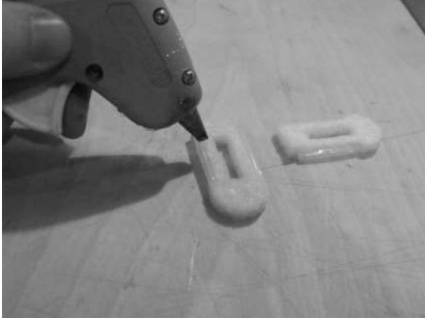
Cut the tube to 1" lengths. Slide the tube to the rounded side of the foam. The tubes should be recessed from the leading edge side to allow motor angle changes. Start by gluing the tube to the foam with both parts laying flat on the table. The tubes will be offset when compared to the thickness of the foam. If not running a motor with a 28mm mounting pattern, adjust this step to accommodate your setup.
