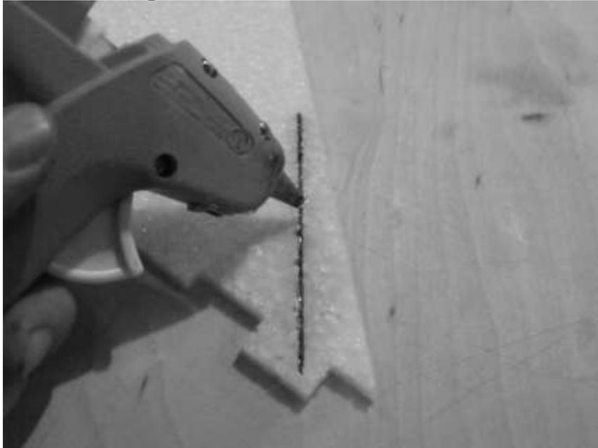
Low temp hot glue works well for this. Insert the carbon and run the glue gun across. The carbon will recess some while doing this. Flip over and do the same, the carbon should be somewhat centered and secured at this point.
