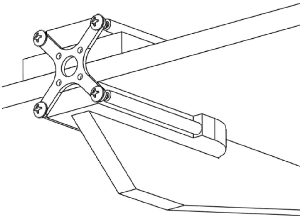
Slide a mount piece onto the foam piece with the long tab. Then slide the tab thru the slot in the body in the front of the plane. A small notch should be cut into the foam to add clearance for the carbon tube near the leading edge.
