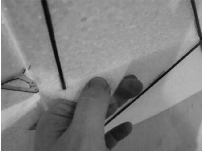
Start by rotating the aft portion of the vertical stab thru the hole, pulling it over the rear carbon spar. With the vertical stab pulled thru enough the forward side will come thru the slot. You can then slide the leading edge of the vertical stab into it's notch.
