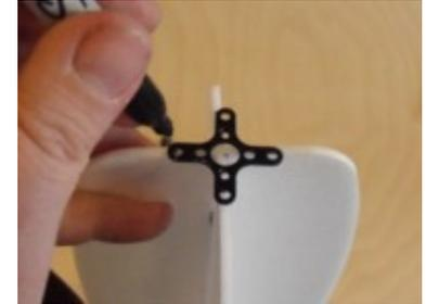
14) **Glue Fuse Nose Bracing** Test fit to underside of fuse, longer end goes up, mounts flush to front of fuse. Beveling the nose braces will increase bonding area (optional).
