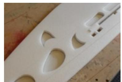
First you can use a light color marker to trace the open areas in the fuse onto the outer panels, these areas will not need glue. Then in the
